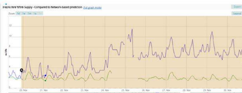
The "hidden leak" (the hidden leak event) continued to show a flow increase even though repair teams were sent to the area, discovered two different leaks, and fixed them.
