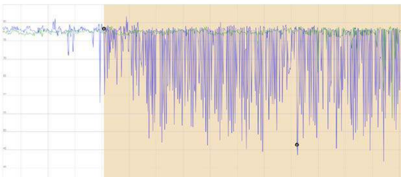
Graph showing the start of the "the pressure decrease event" in TaKaDu.
